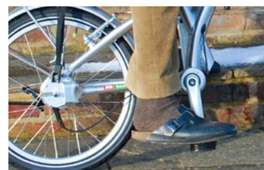
Shaft drive is clean and tidy but is much less efficient than a bush-roller chain
