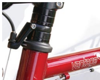
Brake adjusters are sometimes missing from budget tourers. The Vantage has them
