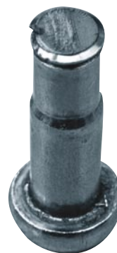
This single saddle bolt sheared off without warning
