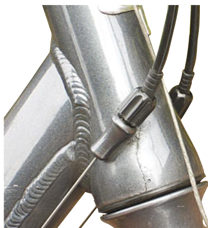
A head tube crack like this is serious. Do not ride a bike in this condition
