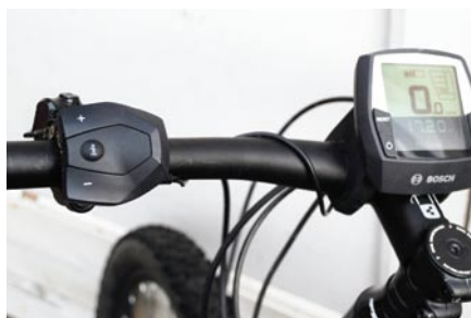
● The left-hand control sets power assistance, while the display shows – among other things – power remaining
