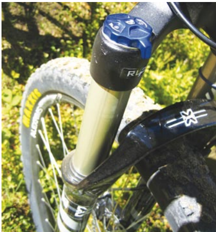
● (Above) Sizes 17.5in and larger get a 100mm fork. The 16in has an 80mm fork so the handlebar isn't too high (Below) Both bikes use a clutch-equipped rear derailleur, which doesn't swing about over bumps
