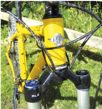
● (Above) A 44mm head tube adds stiffness and maximises fork steerer compatibility (Below) 27.5 isn't a misnomer with this chunky Ardent, but it's only 25mm bigger and 38mm smaller than 26in/29in
