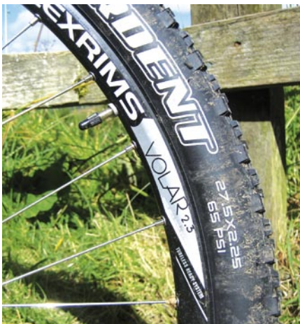
● (Above) A 44mm head tube adds stiffness and maximises fork steerer compatibility (Below) 27.5 isn't a misnomer with this chunky Ardent, but it's only 25mm bigger and 38mm smaller than 26in/29in
