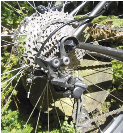
● (Above) Sizes 17.5in and larger get a 100mm fork. The 16in has an 80mm fork so the handlebar isn't too high (Below) Both bikes use a clutch-equipped rear derailleur, which doesn't swing about over bumps
