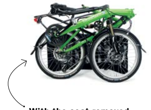
With the seat removed and the frame folded, the Grasshopper fx measures 96x50x70cm
