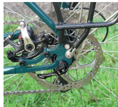
Top: Sora STI levers give convenient shifting but somewhat limit lower gears. Smaller chainrings are an option – and Spa stock them Bottom: The short-pull version of TRP's dual-piston calliper
