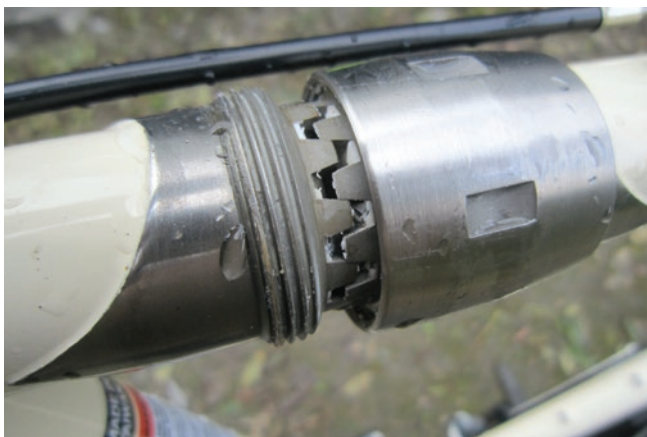
Clockwise from left: The separated joints need to be kept clean. There's no loss of strength or stiffness at the joint. Dropouts allow singlespeed or hub gear use
