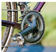
Top: Shimano Tiagra won't work with a large cassette – not unless you were to fit a derailleur hanger extender such as Wolf Tooth's RoadLink Bottom: With only an 11-32 cassette, the 50-39-30 chainset yields huge gears
