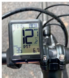
Above: The PulsarOne display shows assistance mode and charge remaining much more clearly than the iWoc controller
