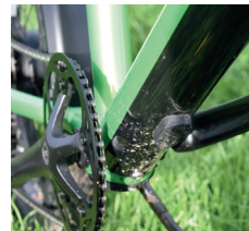
Above: The charging port is fiddly to access and in the firing line from wheel spray
